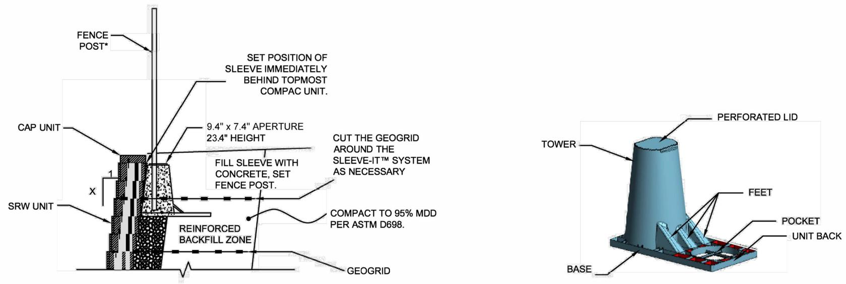
**DETAIL OF FENCE POST INSTALLATION USING SLEEVE-IT™**
