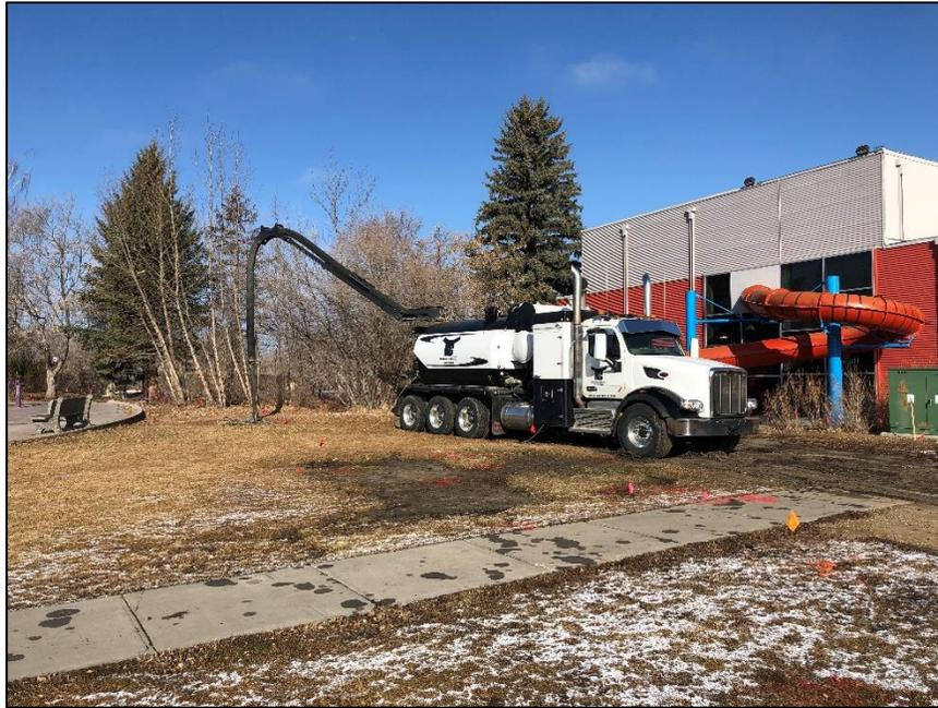
Photo 1: Hydrovac truck setting up for hydrovaccing of location 3.
